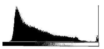
Figure 5. Histogram of the Gray Channel of the Image at 133 lpi Screen Ruling with Round Screen
