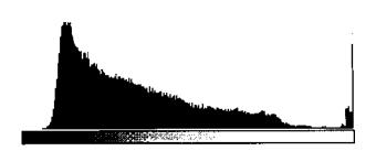
Figure 1. Histogram of the Gray Channel of the Image at 85 lpi Screen Ruling with Line Screen
